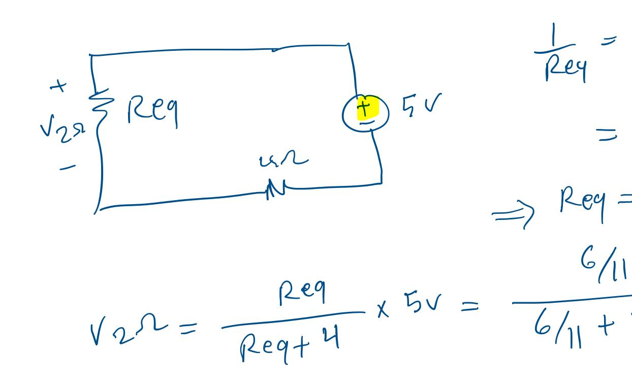
$$\frac{1}{R_{eq}} = \frac{1}{1\Omega} + \frac{1}{2\Omega} + \frac{1}{3\Omega} = \frac{6+3+2}{6} = \frac{11}{6} \Rightarrow R_{eq} = \frac{6}{11} \Omega$$
