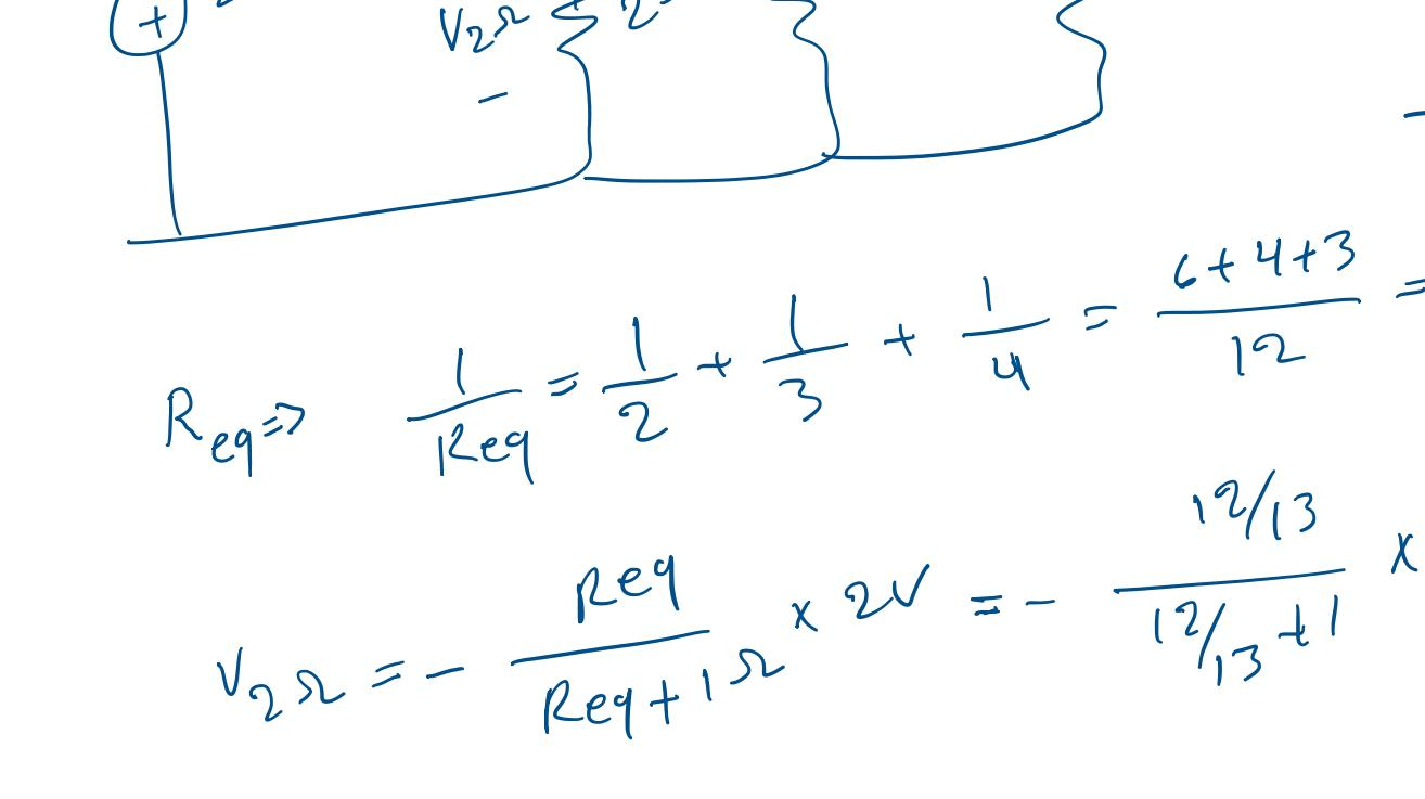
$$R_{eq} \Rightarrow \frac{1}{R_{eq}} = \frac{1}{2} + \frac{1}{3} + \frac{1}{4} = \frac{6+4+3}{12} = \frac{13}{12} \Rightarrow R_{eq} = \frac{12}{13} \Omega$$
